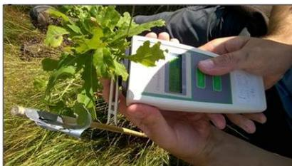
using a photosynthesis analyser to measure stress
