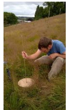
using a drop disk to measure the height of ground flora
